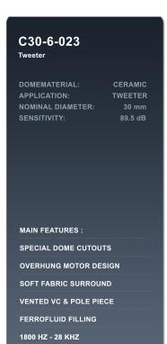
The C30 - 6 - 023 is a 1.2 inch tweeter with ultra hard ceramic dome in a 106 mm frontplate.
